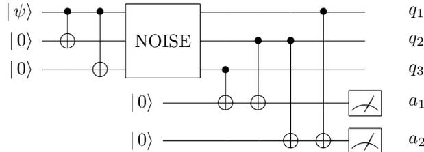
Verify that we can detect a single bit-flip from the noisy channel by measuring the two ancilla qubits ( $a_1$  and  $a_2$ ) in the computational basis  $\{0, 1\}$ . Specify what corrections would be required for each possible measurement result.
